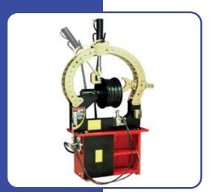
Basic/medium Straightener with double electro hydraulic cylinders and all around bridge. The best option for mobile wheel repair shops or shops where just 110V single phase electricity is available. Fixes wheels up to 24"
